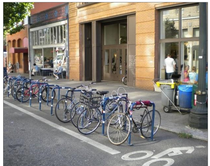
Required bicycle storage racks shall be within 100 feet walking distance of the project's main entrance.
